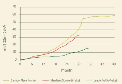
**Figure 1:** Construction waste generated by off-site and in-situ construction (measured in cubic metres of waste per 100 square metres of gross internal floor area (GIFA))
